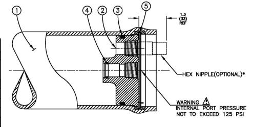
WILL CAUSE SEVERE LOCAL STRESS AROUND PORT AND MAY RESULT IN LEAKS AND PREMATURE FAILURE; TAKE EVERY PRECAUTION LISTED ON PAGE 02, SEE INSTALLATION INSTRUCTIONS FOR FURTHER DETAILS
